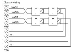
Marking indicates output signal polarity when the circuit is active. Polarity reverses when the circuit is not active. Wire notification appliances accordingly. Notification appliance polarity shown in active state.
