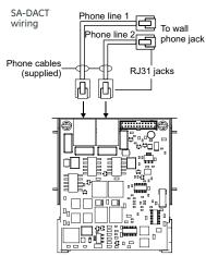
The dialer phone lines connect to connectors on the dialer's main circuit board. Phone line 1 connects to connector J4 and phone line 2 connects to connector J1. The SA-DACT queues messages and transmits them based on priority (alarm, supervisory, trouble, and monitor). Activations are transmitted before restorations.
