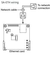
The SA-ETH card provides a standard 10/100 Base T Ethernet network connection for connecting to an intranet, a local network, or the Internet. The card can be used to download configuration programming from the VS-CU to the panel over the network.
