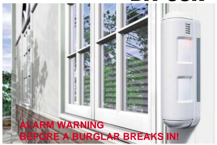
Outdoor PIR Protection that covers a building's perimeter: the BX-80N's long, narrow detection area comes from the centre point, covering both sides.
